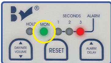
**G** Place individual in bed. The yellow HOLD light will flash for 5 seconds, then beep once as green MON light illuminates – the individual is being monitored. To immediately monitor, press RESET once. **Verify MON light is on before leaving individual unattended.**
