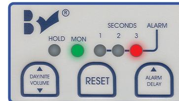
**J** If the individual has not been removed from the bed or chair within 25 seconds **after pressing RESET**, the control unit will return to the green MON (monitor) mode **automatically**. **NOTE:** Instantly go from MON to HOLD or from HOLD to MON by pressing RESET.
