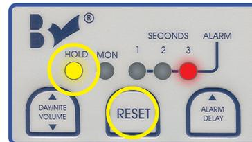
**I** To remove the individual from the bed or chair **without the alarm sounding**, press RESET. The yellow HOLD light will flash. Now assist individual from the bed or chair. The control unit remains in HOLD until weight returns to the Sensormat pad.
