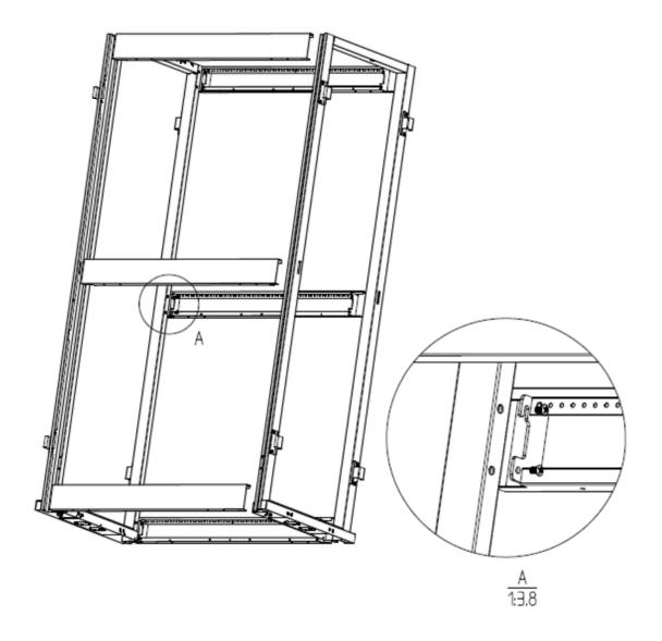
Parts name: Front frame\* 1 pcs ; Back fram\*1 pcs Support beam\*6 pcs; M6\*12 thumb Screws\*24 sets
