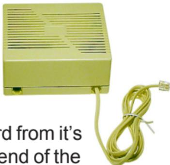
Unplug the telephone's line-cord from its wall-socket and plug the other end of the supplied lead into the telephone's wall-socket (the one that you've just removed the telephone's line-cord from).
