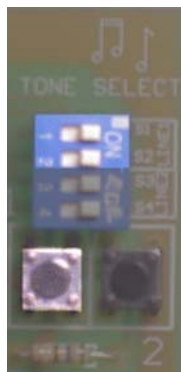
Line 1 Tone selection switches and test button
