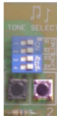
Line 2 Tone selection switches and test button
