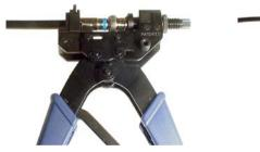
Place the cable and connector into the laws of the crimp tool, passing the cable into the "v-notch" at the left-handside of the tool.
