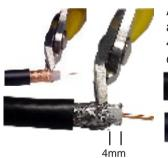
A) Remove the dielectric and shield from the last 4mm to expose the inner conductor.
