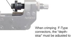
When crimping Female BNC or Female F-Type connectors, the "Flat-nut" is used and the "depth-stop" is adjusted to position "3".
