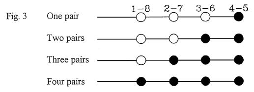
If the cable is a wired straight-thru, the LEDs will illuminate green. If it is reverse wired, the LEDs will illuminate red.
